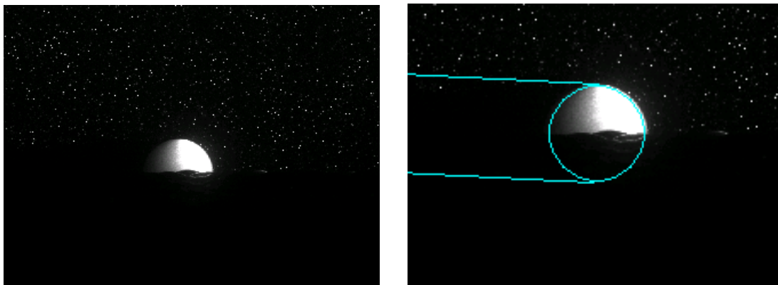
Figure 7-12 (Cam2, Run E, Delrin) Image of particle settled in the flow bottom at his protrusion before entrainment, on the right the same particle after the particle detection, showing with the blue lines the target sediment and an area behind it for limiting the shadow flow field.
