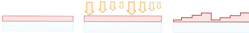
Figure 1.2: the three main step of mask-less lithography: photoresist coating, exposure, development of the final structure.
