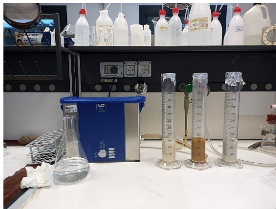
Figure 43 Sample before and after 24 hour with a clear differentiation of the binder fraction
