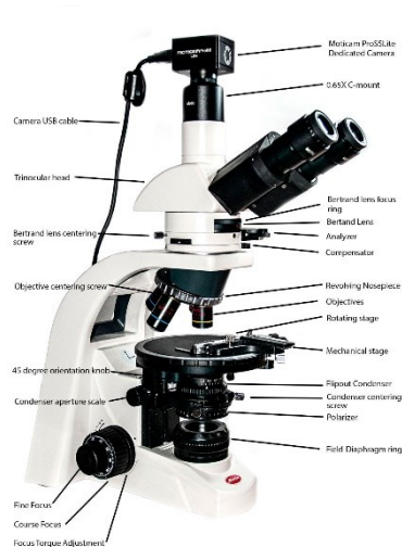
Figure 32. Typical aspect of a polarizing optical microscope.
