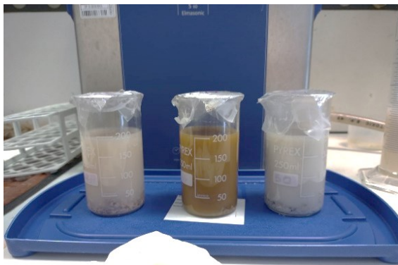
Figure 43 Sample before and after 24 hour with a clear differentiation of the binder fraction
