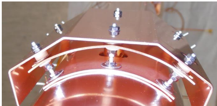
Figure 3-13: Unshielded pickup, used as trigger or photon pickup.
