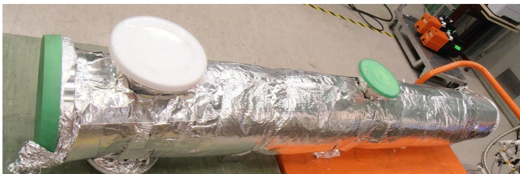
Figure 7-19: Bake out jacket for a chamber.
