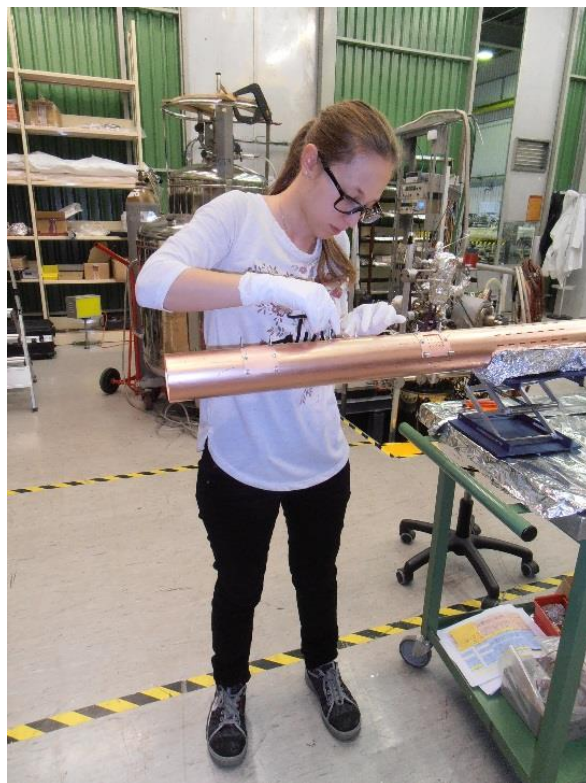
Figure 7-16: me mounting the pickup and calorimeters on liner in b. 113.
