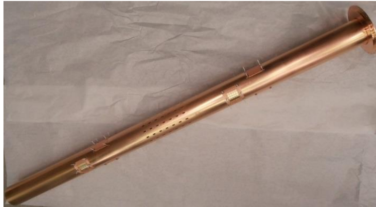
Figure 3-7: VPS liner with windows for pick up and calorimeters.
