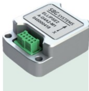
Figure 3.32: Ellipse 2 Micro AHRS (dimensions :26.8 x 18.8 x 9.5 mm 3 ; weight : 10
