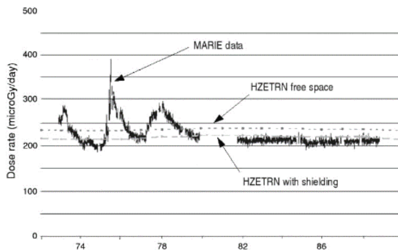
Figure 2.9: Radiation dose-rate at Mars as measured by MARIE and as calculated using HZETRN for March 2002
