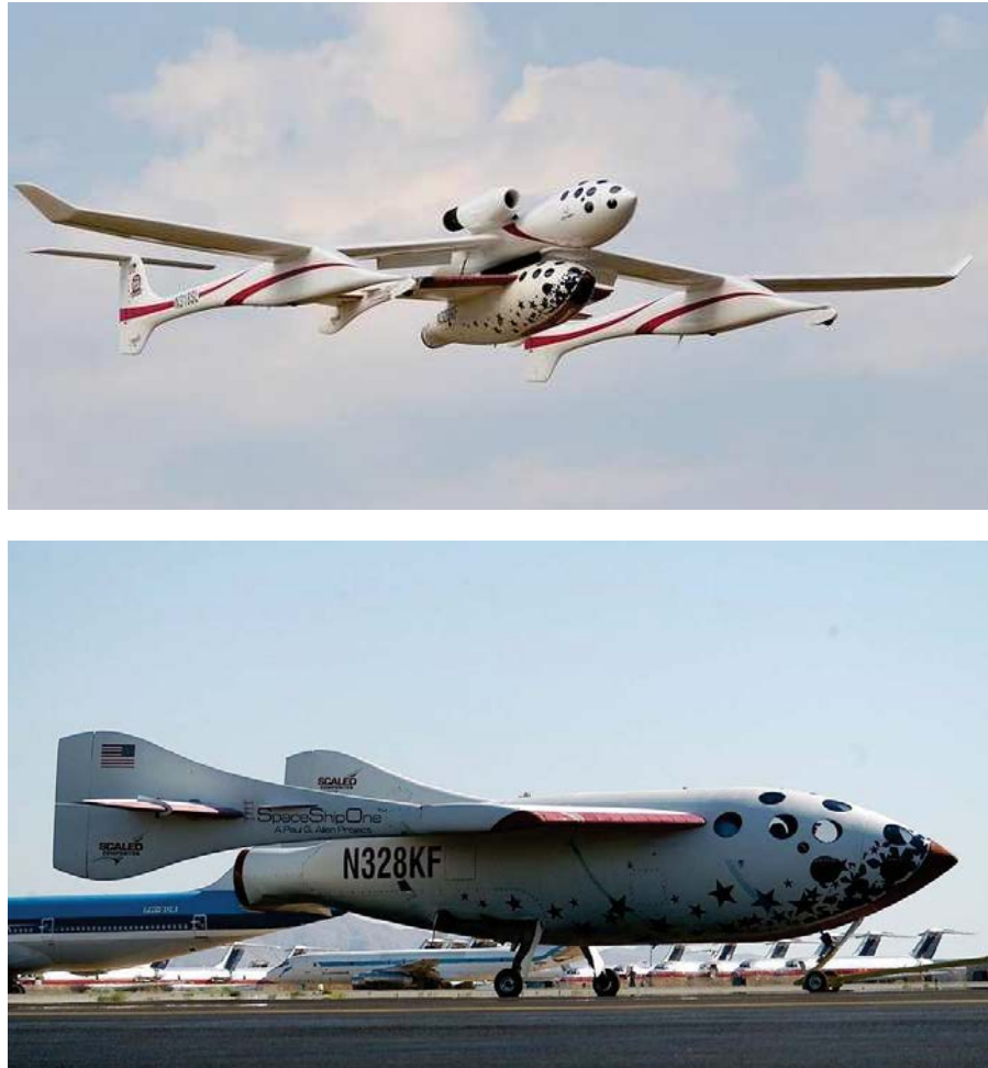
Figure 1.10. SpaceShipOne and White Knight carrier.
