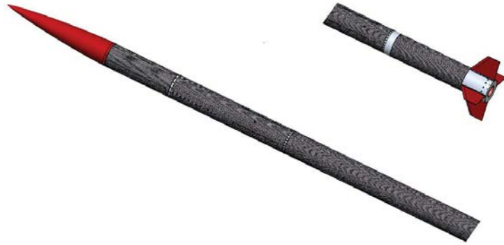
Figure 5.18. Upper and Lower parts of the rocket after the FTS activation.
