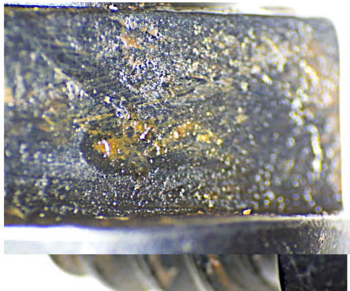
Figure 23 Threads of the screw showing only surface debris and no damage to the bluing.
