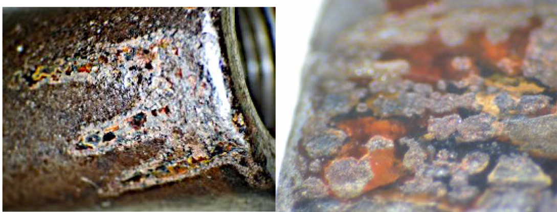
Figure 20 Severe erosion to the exterior side of the breech block(left), with the formation of various coloured patinas and similar patinas on the interior side (right).
