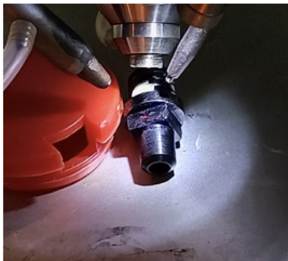
appendix 1 Lock plate under XRF.
