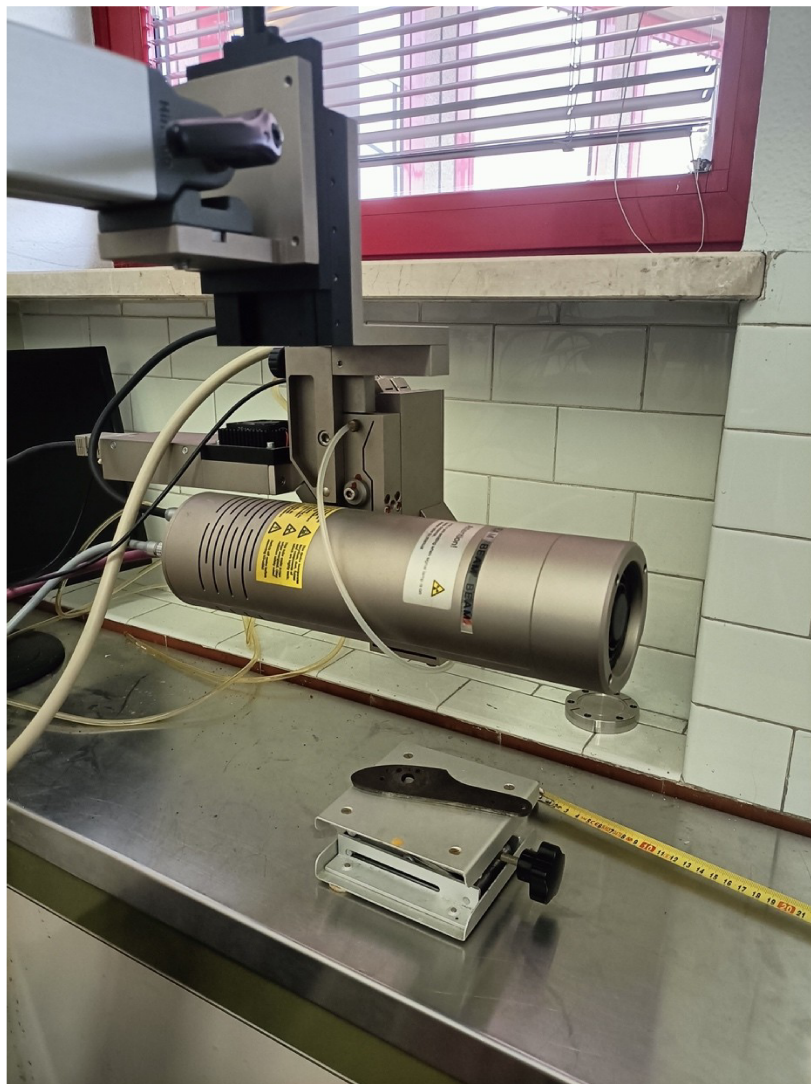
Figure 12 The XRF set up with the lock plate in position.
