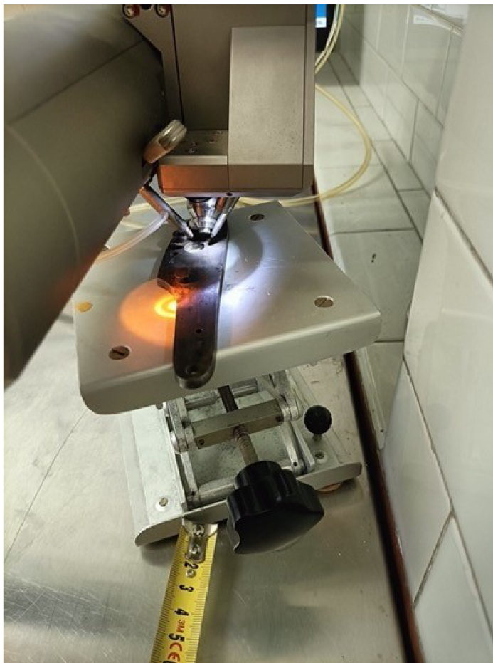
appendix 1 Lock plate under XRF.
