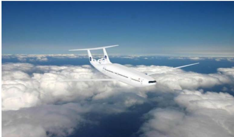
FIGURE 2.14: D8 Double Bubble concept developed within NASA N+3 project [35]
