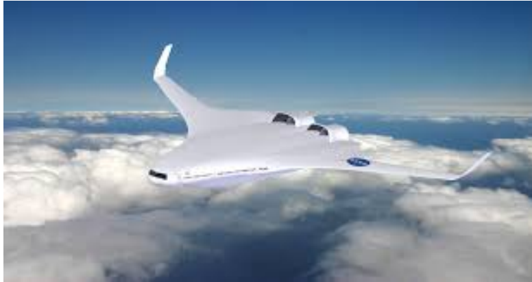
FIGURE 2.16: Conceptual design for BWB H3.4 configuration [36]
