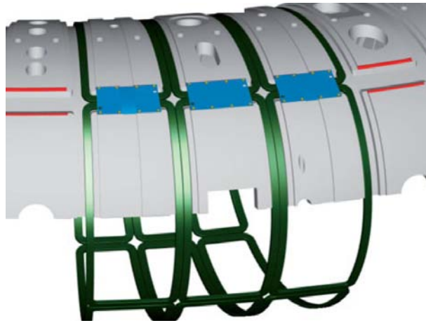
Figure 3.4: The saddle coils mounted around a torus section [15].
