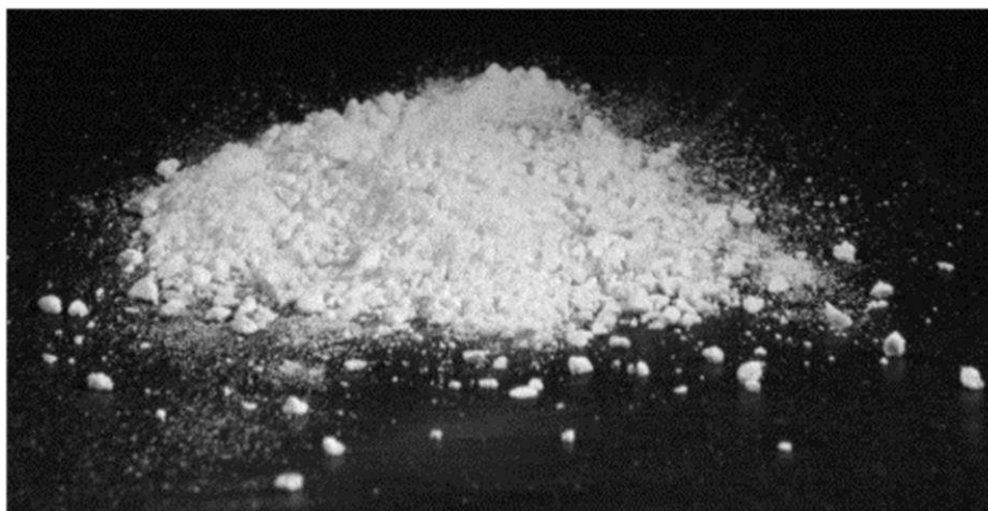
Figure 2.13 - Granules produced after the milling of a test batch of ribbons with an average porosity equal to 36.2%
