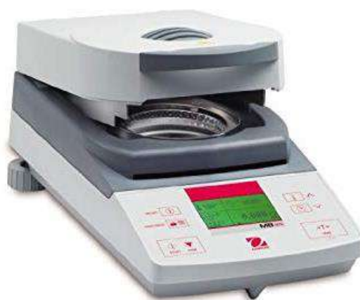
Figure 2.9 - OHAUS® MB 35 Moisture analyser used to determine the moisture content of the powder [69]
