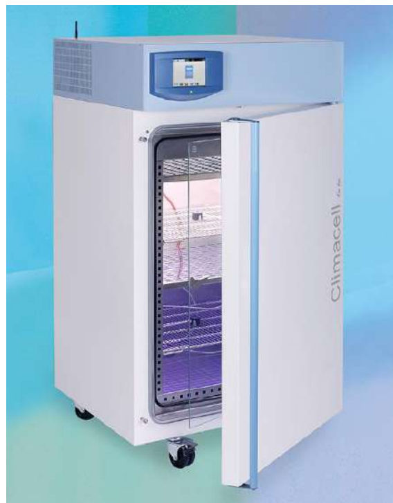
Figure 2.8 - Humidity chamber CLIMACELL™ used to perform the experimental study of the humidity effect in the powder behaviour [9-W]
