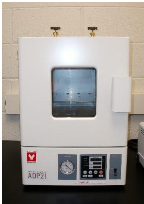
Figure 4.1: Yamato ADP 21 Vacuum Drying Oven
