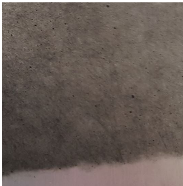
Figure 4.23: Non dense fibers collected on the Aluminum foil
