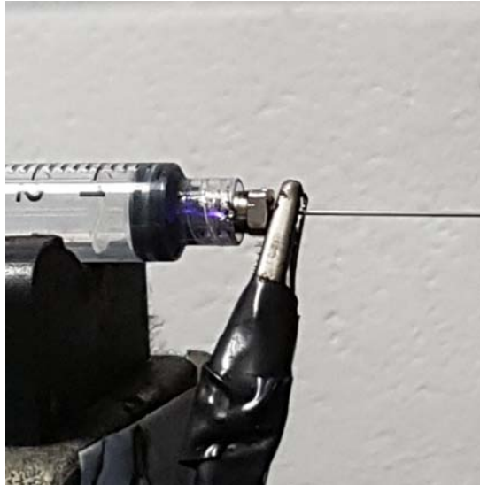
Figure 4.15: Example of sparks inside the syringe
