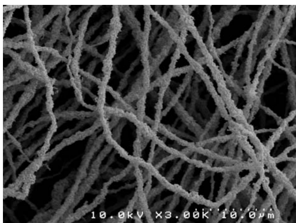
Figure 4.24: SEM image of water/IPA/MeOH fibers
