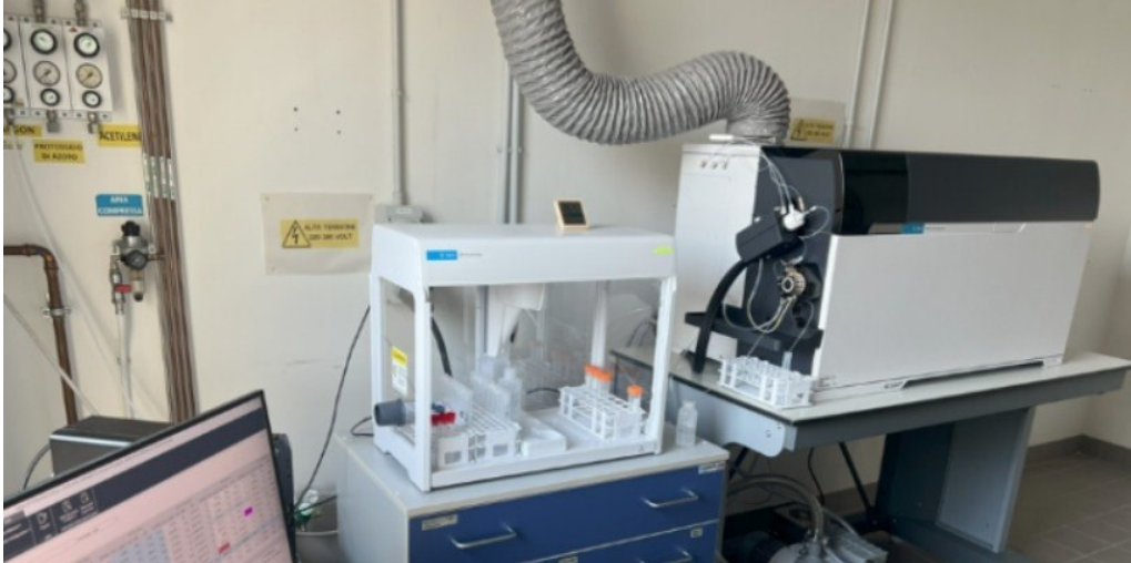
Figure 11 ICP-MS instrument used for the analysis of liquid samples at the Department of Geosciences, University of Padova.
