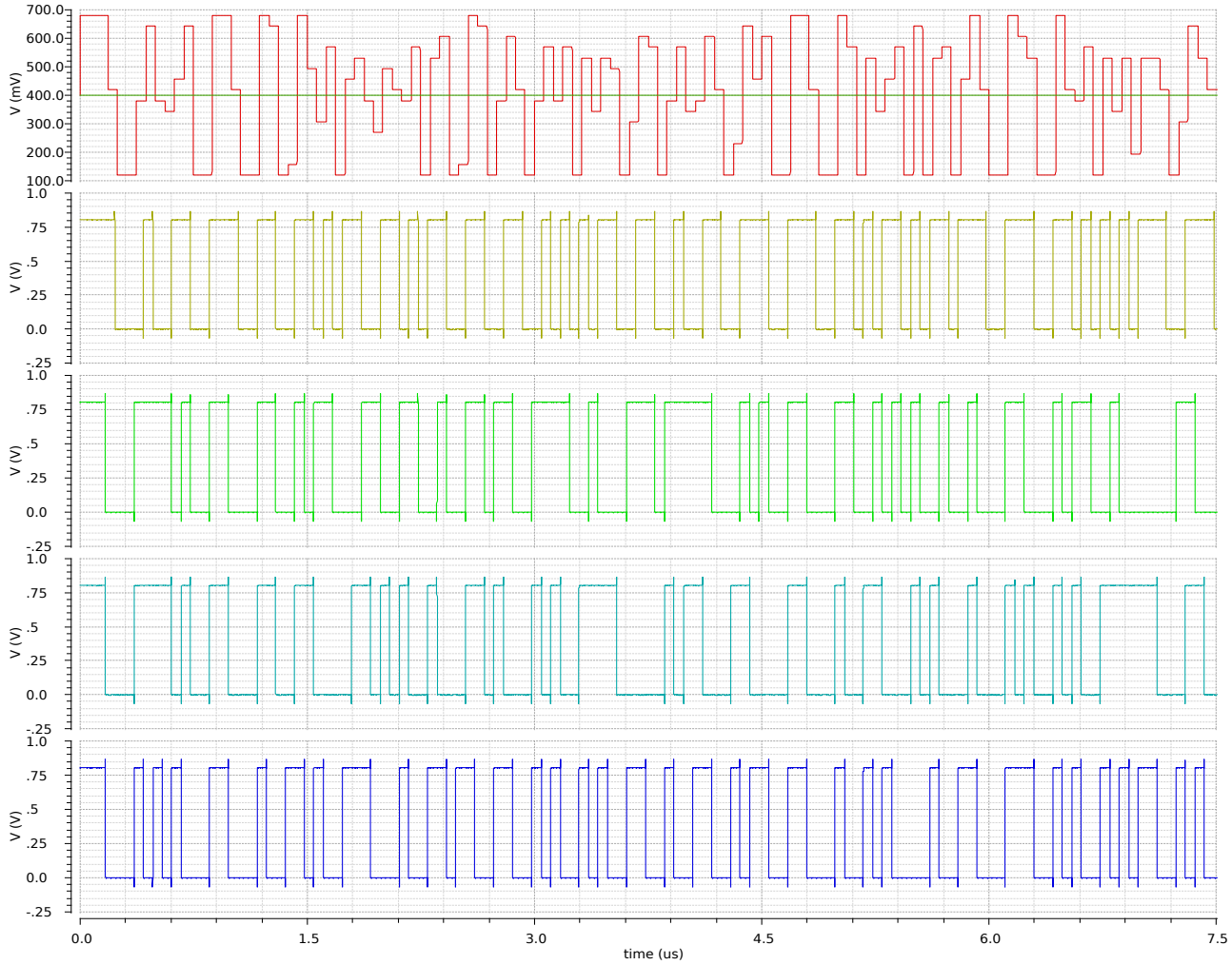
Figure 4.15: Modulator's output with SAR quantizer in post layout simulation showing the modulator output and zero input(only common mode voltage) and then the 4 output bits
