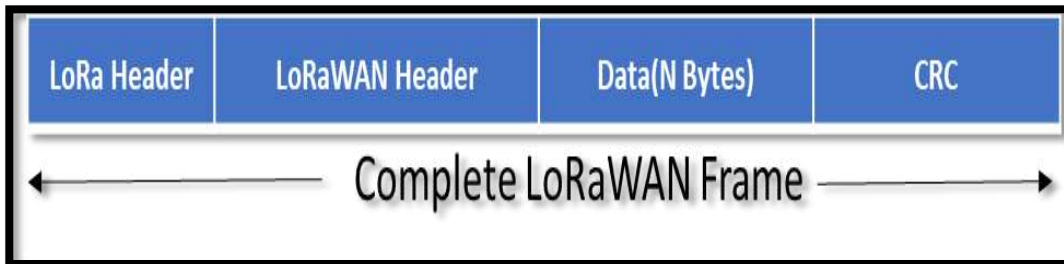
Figure 16: LoRaWAN Simple Packet format.
