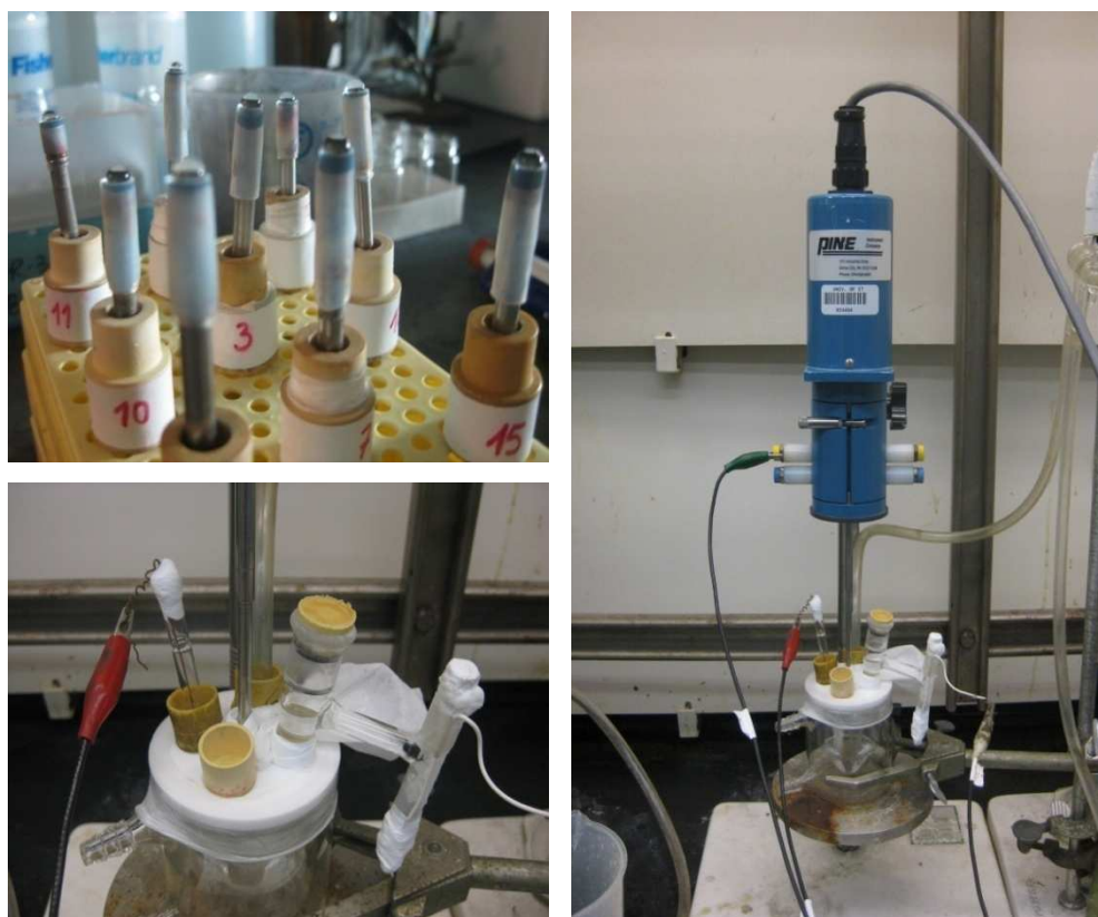
Figure 21. In the upper image, there are the electrodes during the incubation of Ab_1 . On the right, the rotating disk electrode system is represented entirely, and in the last image there is a zoom of the electrochemical 5 holes cell that we used for the measurements.
