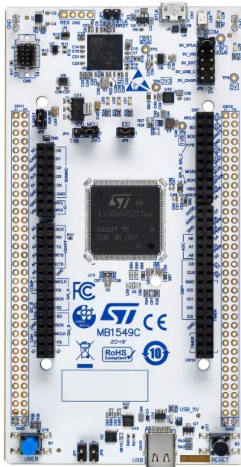
Figure 27 - NUCLEO-U575ZI-Q development board used for the payload DM.
