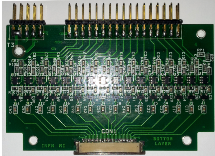
Figure 3.3: Preamplifier board for the \Delta E stage electronics. Each board handles 16 lines. In the upper side there are the biasing connector (left) and the signal connector (central). Board dimension: 78 \times 47 \text{ mm}^2 .
