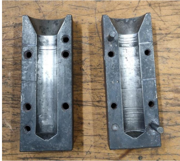
Fig. 3.1: The cleaned die used for the casting process
