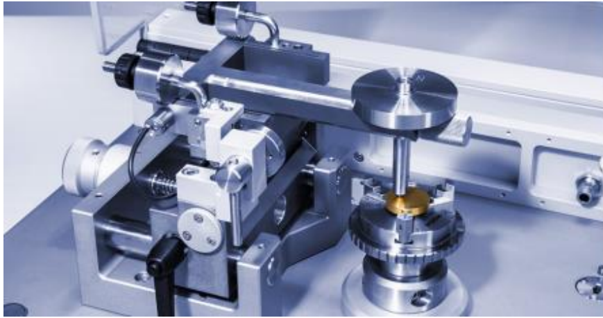
Fig. 4.16: The tribometer used for the wear test [20]
