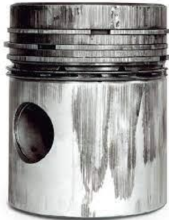
Fig. 1.5: Wear rate effects on a piston [5]
