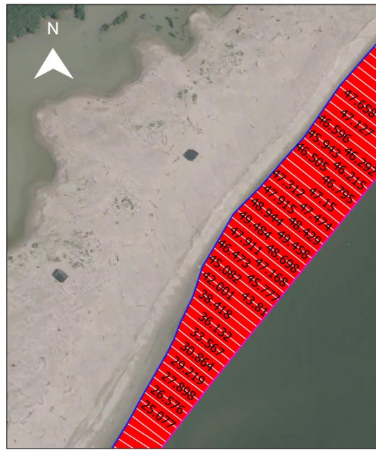
Figure 91 Central part of cell RO10 with indication of perpendicular distances between coastlines, 2015 orthophoto.
