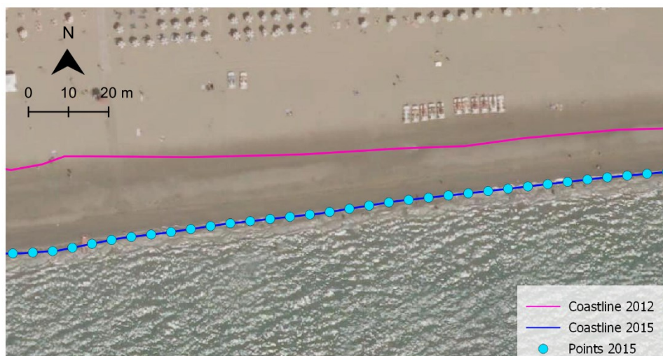
Figure 22 Points placed every 5 m on coastline 2015 (Bibione, VE). The orthophoto on the background is taken in 2015.
