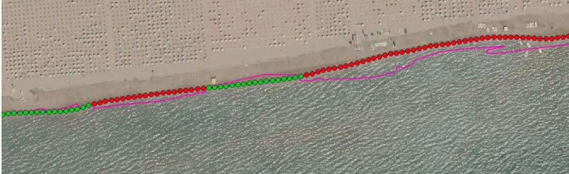
Figure 27 Points along 2015 coastline are colored in order to highlight deposit (green) or erosion (red) zones.
