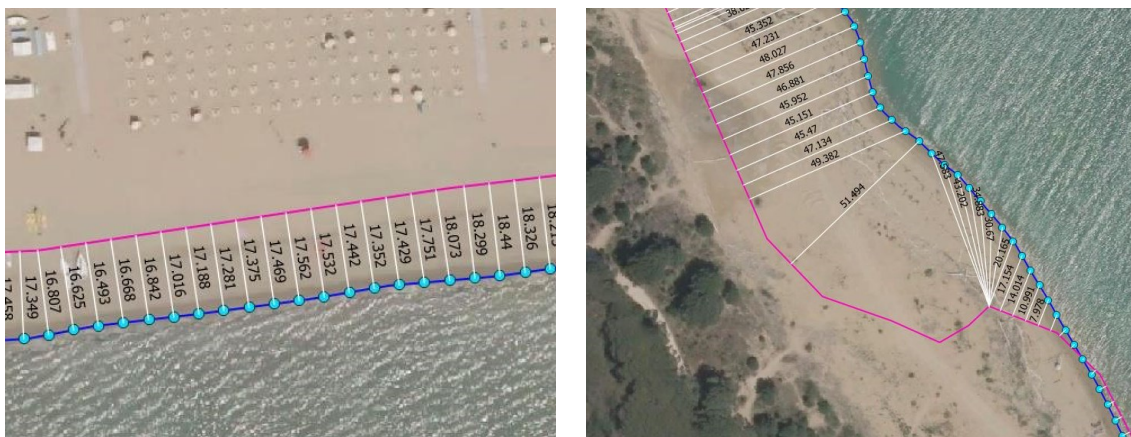
Figure 26 Left: example of good calculation of perpendicular distances between coastlines (Bibione, VE). Right: limits of QGIS application for the calculation of perpendicular distances between coastlines (Bibione, VE).
