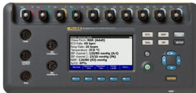
Figura 2.28 - Fluke ProSim 8 Vital Signs and ECG Patient Simulator
