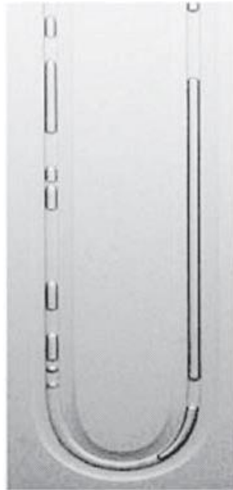
Figure 8 - Slug flow in a bended channel (Khandekar et al. 2003)
