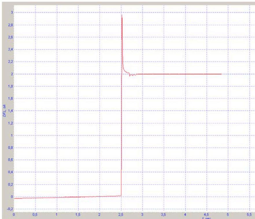
Figure 2.11 Example of approach in a contact-mode AFM.
