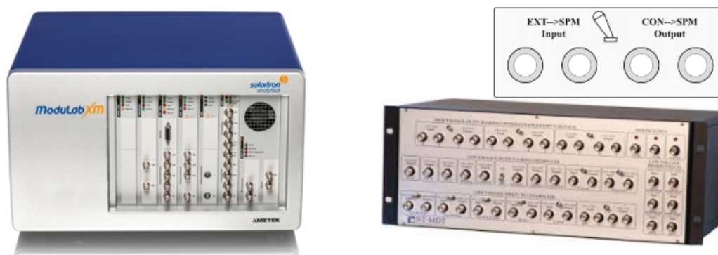
Figure 2.14. Potentiostat ModuLab XM ECS (left) and Signal Access Module SAM01 (right) used coupled with AFM controller for IS-AFM measurements.
