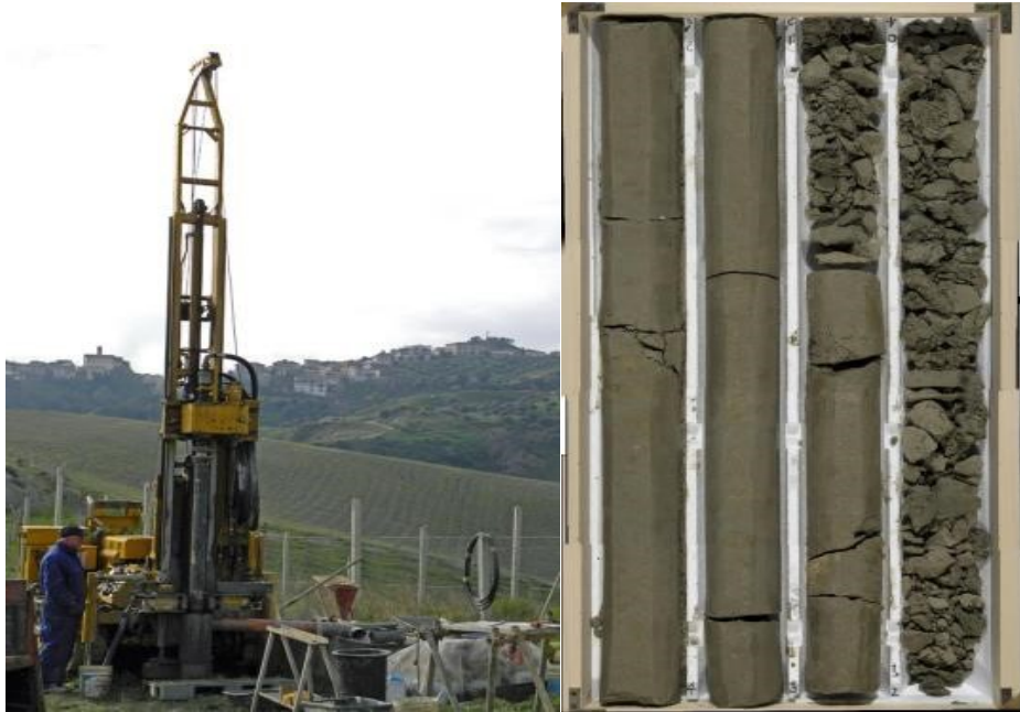
Figure 2.2.4 Left: Caterpillar at work in the Crosia Village. Right: Sediments stored in dedicated polystyrene boxes, with the rightmost core in the box loose and unrepairable.
