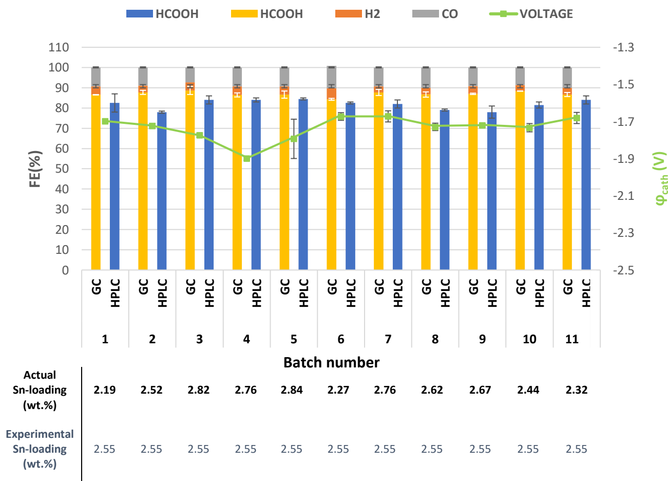
Figure 6.2. Graphical representation of the Faraday Efficiencies for different \text{SnO}_x\text{@AB} batches. Every batch is characterised by two bars, the first was defined through a GC and the second through an HPLC. In the table below, the actual and experimental Sn-loadings (wt.%) are showed per every batch. \text{CD}=-400\text{mA}/\text{cm}^2 ; catholyte= 0.5 \text{K}_2\text{SO}_4 ; T\sim 42^\circ\text{C} ; anolyte=bi-distilled water; t=120 \text{min} at CCE; catholyte volume= 40 \text{mL} ; flow rate= 9 \text{mL}/\text{min} .
