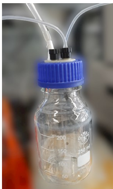
Figure 5.3 Photo of the catholyte reservoir.
