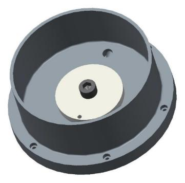
*Figure 22* 3D rendering of the basin assembled with the UHMWPE disc.
