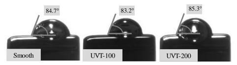
Figure 26 Water droplets on the surfaces of the Ti6Al4V machined samples.
