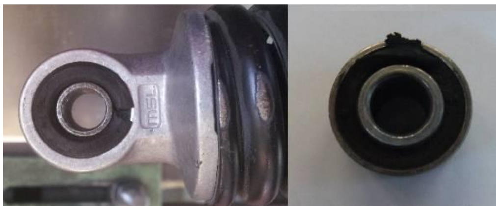
Figure 188 - Rear shock absorber silent-block failure.
