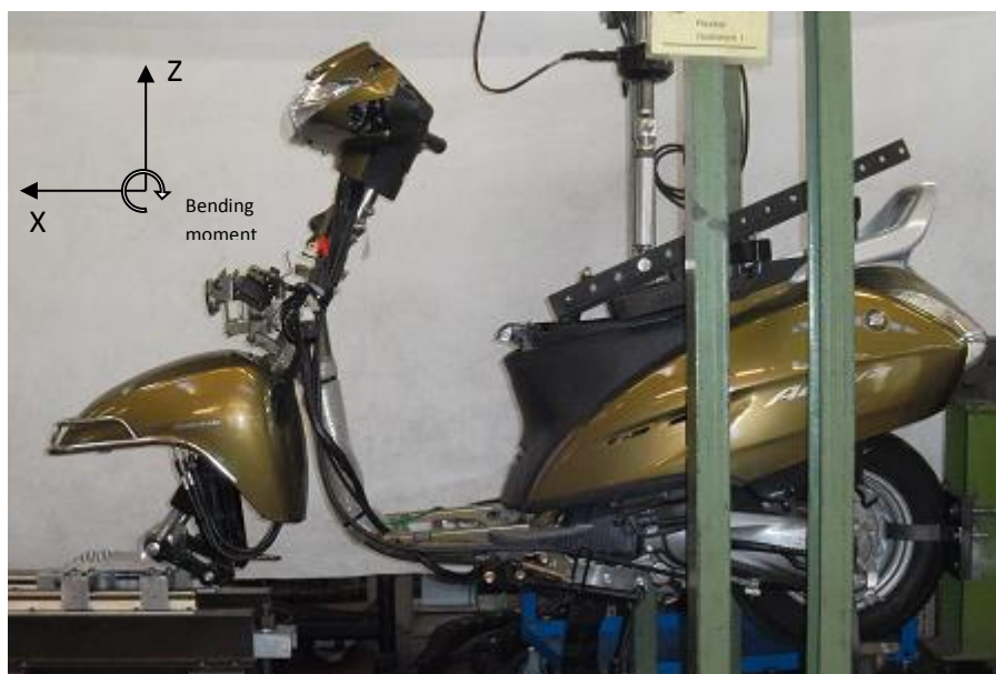
Figure 12 - ActivaD on fatigue test bench.
