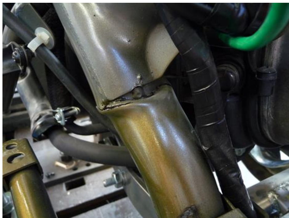
Figure 197 - ActivaD, right weld toe failure at critical point (CPR).
