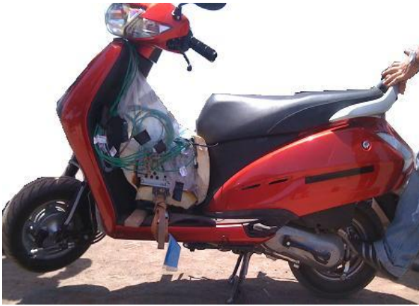
Figure 28 - G0 front condition (zeroing).
