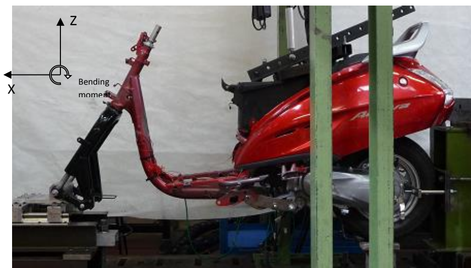
Figure 14 - ActivaD2 on fatigue test bench.
