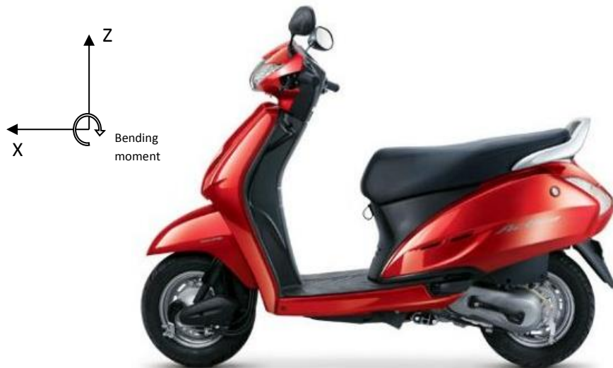
Figure 1 - Honda Activa and data reference system.
