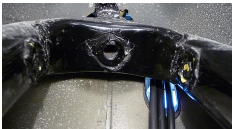
Figure 199 – ActivaD, front fork failure.
