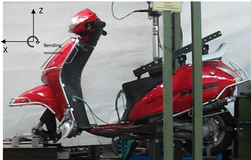
Figure 2 - ActivaS on fatigue test bench.
