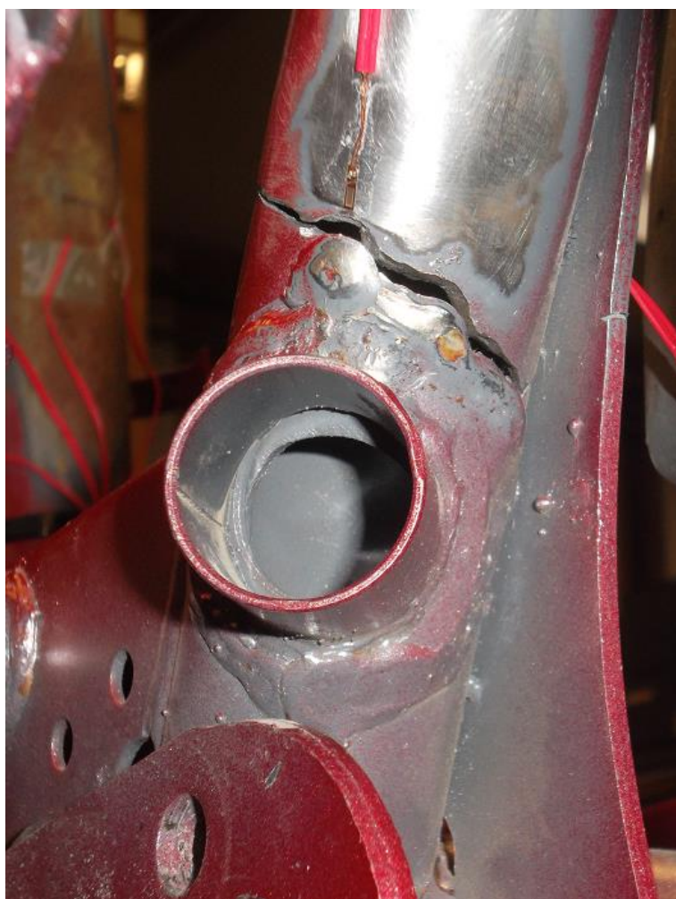
Figure 202 – ActivaD2, left weld bead failure (CPL).
