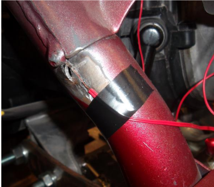
Figure 203 - ActivaD2, right weld bead failure (CPR).
