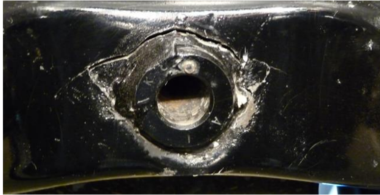
Figure 200 – ActivaD, detail front fork failure.
