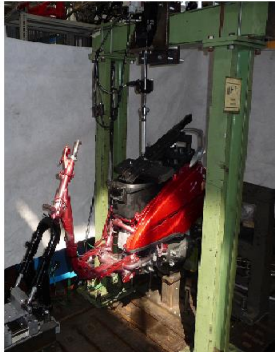
Figure 17 - Test Bench hydraulic piston.
