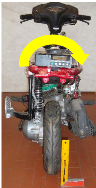
Figure 195 - Overall frame torsional.
