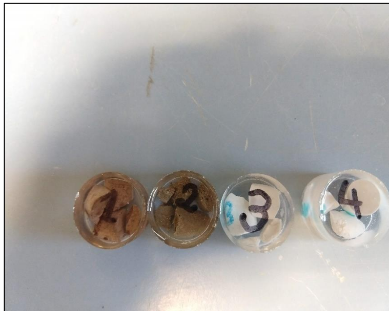
Fig.18: Crushed cylinders samples numbered according the sample name impregnated with epoxy resin before being analysed via SEM.
