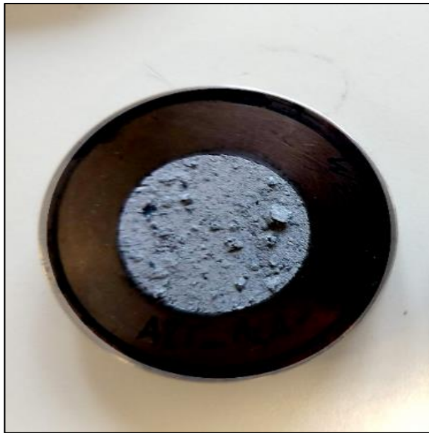
Fig. 60: Sample of fly ash exposed to ambient conditions for 3 days. Swelling is observed.
