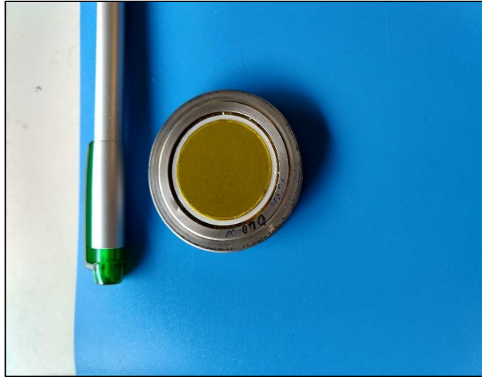
Fig. 21: Sample holder used for kinetic analysis performed on hydrated sample 4. The sample was covered by a Kapton layer.
