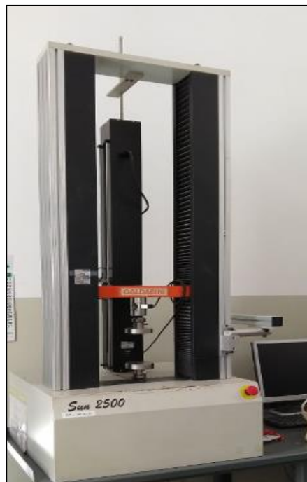
Fig. 23: Material testing machine used during the compressive strength test.
