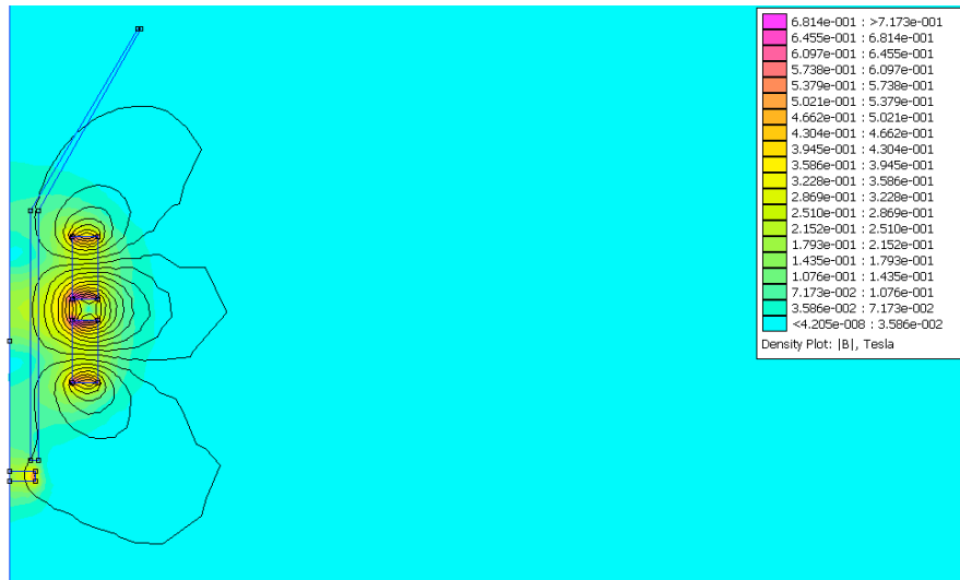
Fig. 5.7: FEMM solver results for the magnetic field configuration reproduced in F3MPIC. In this figure it is possible to appreciate the spatial configuration of the external magnets. The problem has a cylindrical symmetry.
