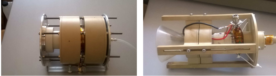
(a) Prototype of the new thruster developed during the STRONG project
