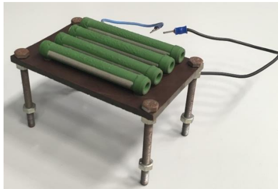
Chapter 1, Figure 19 - The four 5 k \Omega resistors parallel connected and their sustaining structure.
