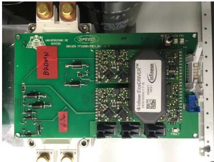
Chapter 1, Figure 3 - The driver by Infineon is located on the top of the electronic board on which it is possible to recognize: 3 optical fibre gates, the fault led, the blue 6 pins terminal (sending errors to the DSP), the white power feeding terminal, 2 feeding checking led and the button to reset the error signal. The white plastic object with 4 bolts, that lies under the driver, is the power module.
