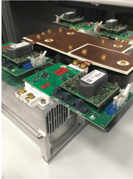
Chapter 1, Figure 2 - The picture of the whole 3P4L inverter completely mounted.
