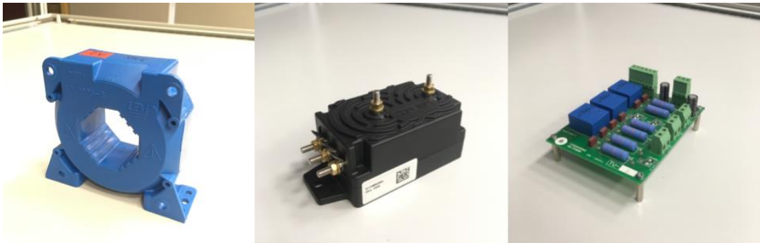
Chapter 1, Figure 15 - From left to right: current sensor, DC-bus voltage sensor, electronic board with three voltage sensors.
