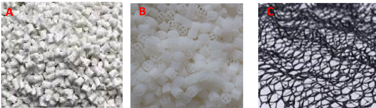
Fig. 15 A Filling material VALOX – Fig. 15 B Filling material KALDNESS – Fig.15 C Filling material GEOMAT
