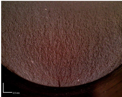
(c) Fatigue lines in part of the fracture section with 57.2x magnification
