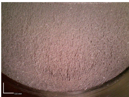
(c) Fatigue lines in part of the fracture section with 63.1x magnification
