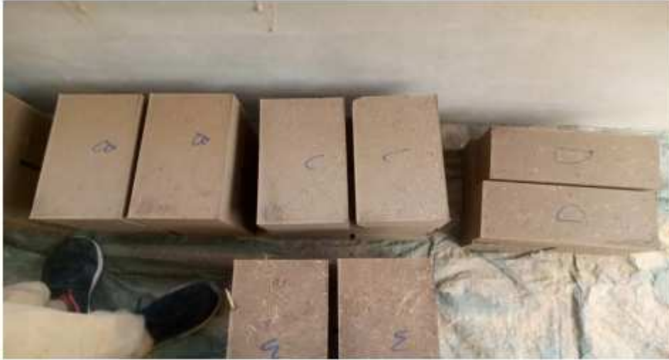
Picture 3: Compressed stabilised mud brick samples
