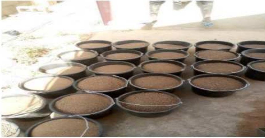
Picture 2: Soil proportioning for mixing
