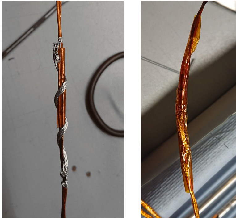
Figure 6.2: Wires ready for the vacuum, appropriately shielded and tinned.
