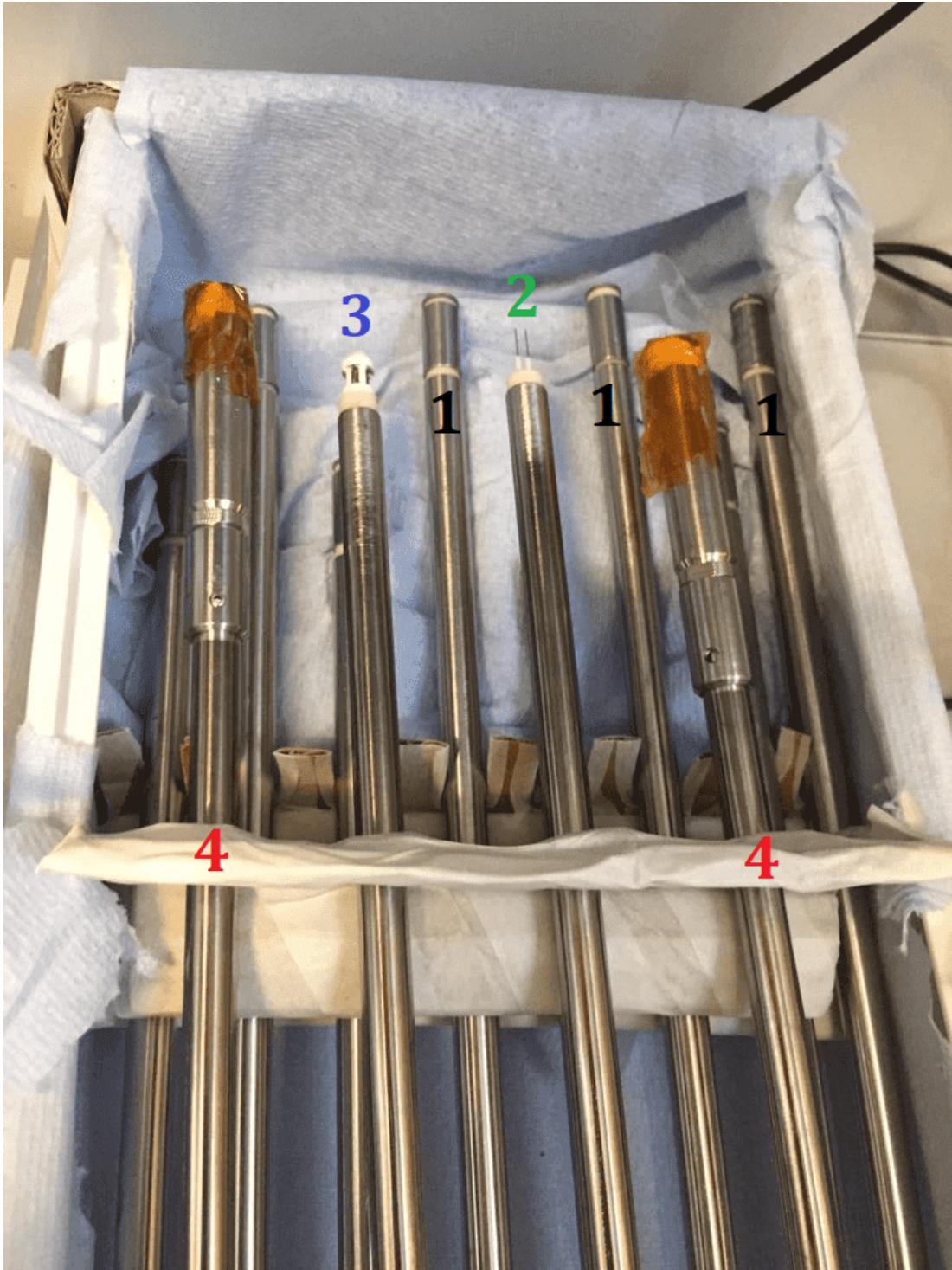
Figure 6.1: All the probes used assembled on their support. The planar probes are marked with a black 1, the double probe with a blue 2, the Mach probe with a blue 3, the RFEAs with a red 4.
