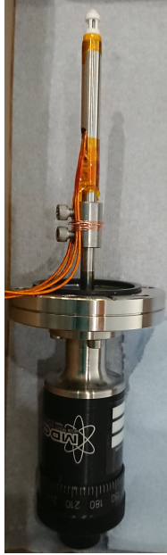
Figure 3.22: New rotating system, assembled with the new probe.
