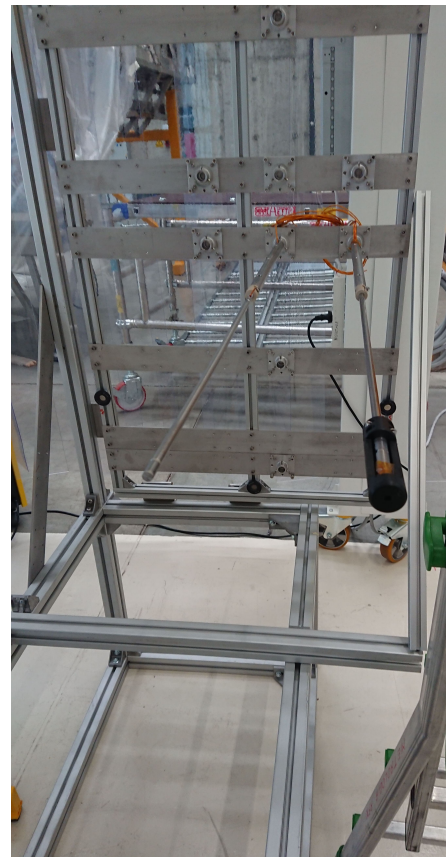
Figure 6.4: The framework which will be used as support inside SPIDER with two probes ready.
