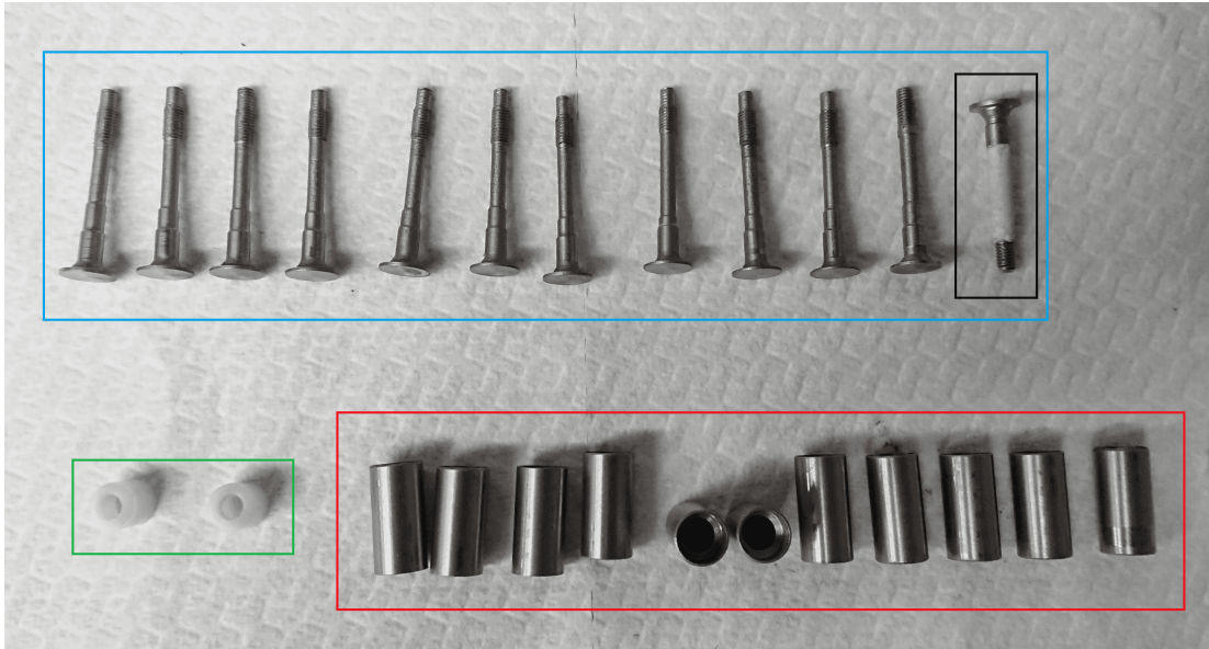
Figure 5.1: Langmuir probe components ready to be assembled.
