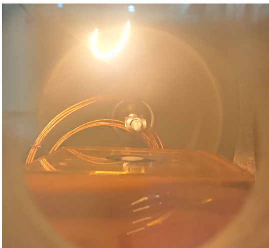
Figure 3.4: Mach probe inside ATHENIS, front view.
