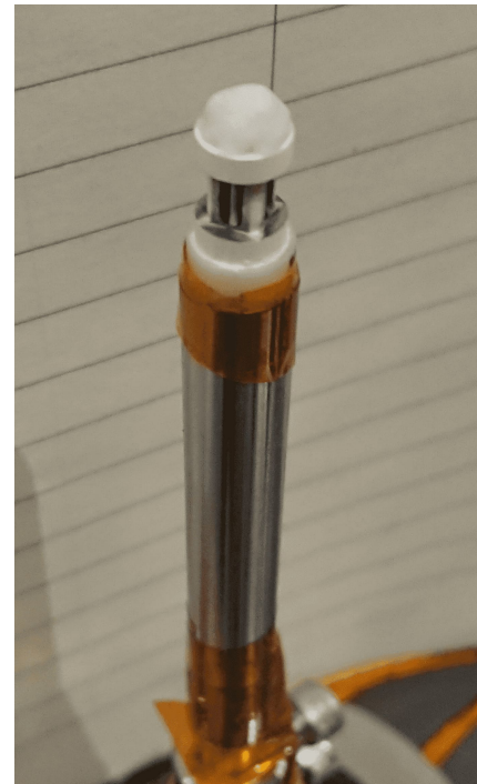
Figure 3.34: Sputtered probe after the measures.
