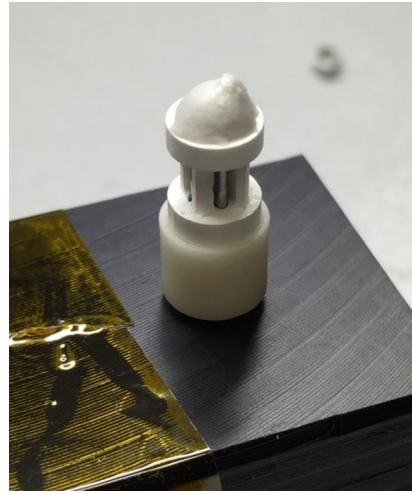
Figure 3.23: New probe tip, with Boron Nitride support and ceramic glue.
