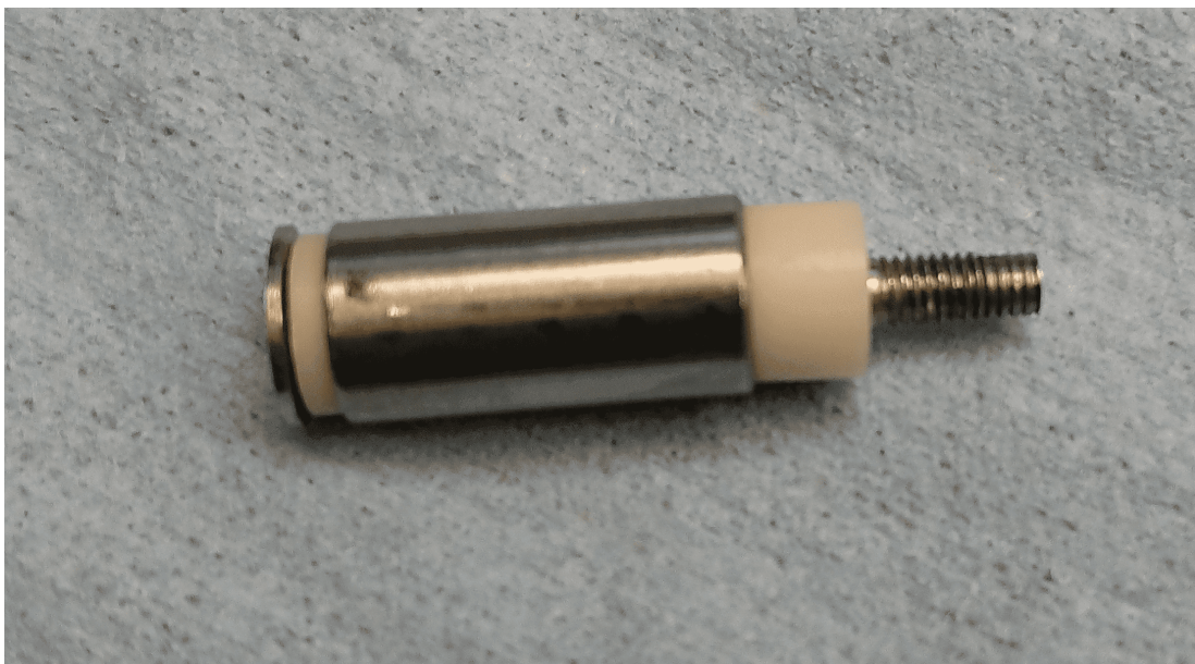
Figure 5.3: Fully assembled Langmuir probe tip.
