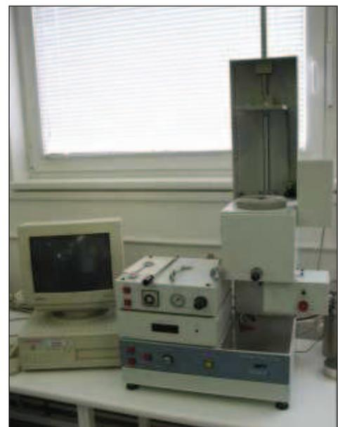
**Figura 2.2: Plastometro Melt Flow Index**
