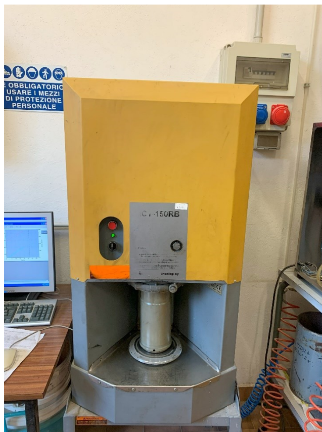
Figura 4.21: Superpave Gyratory Compactor (SGC).
