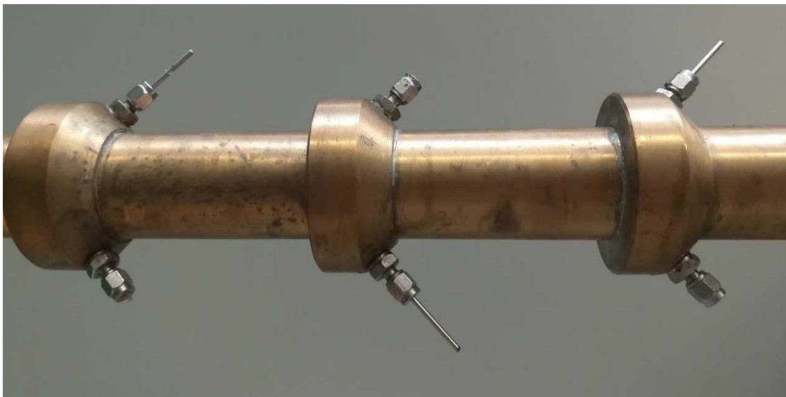
FIGURE 3.5 – RTD SENSORS DISPOSITION ON THE ANNULAR TUBE
