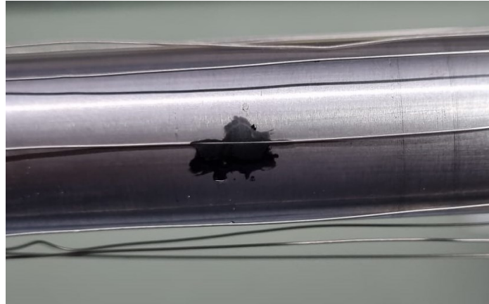
FIGURE 3.11 – DOT OF GLUE APPLIED ON A LOOSE TC.
