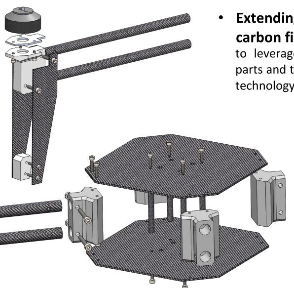
**Extending the concept of 3d printed parts joining** carbon fiber composite tubes or plates
