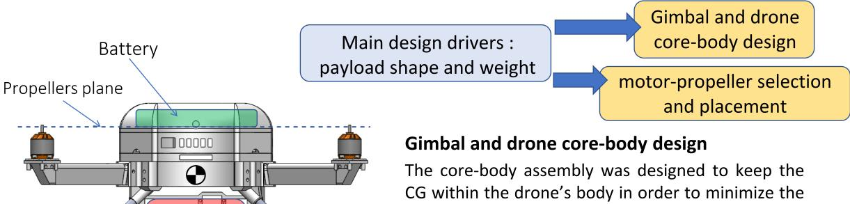
CG within the drone's body in order to minimize the vertical distance between the CG and the center of thrust located on the propeller's plane in favour of stability[1]
