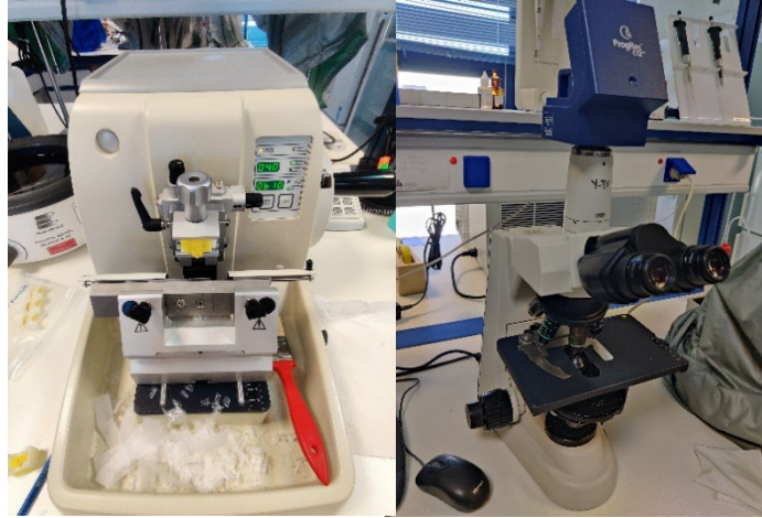
Fig. 7: semi-automatic microtome (Leica RM2245, Germany), light microscope (50i Eclipse, Nikon, Japan) with digital camera (Progres, Jenoptik AG, Germany)
