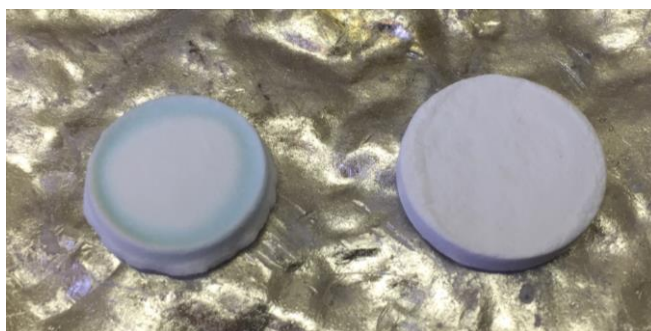
Figura 3.5 Pastiglie 80%PDS - 20%Biosilicate® e 60%PDS - 40%Biosilicate®.
