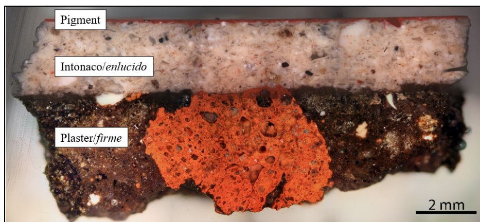
Figure 28: Darkfield micrograph in reflected light of sample 6Pi1 in cross-section, indicating the pigment, intonaco, and base plaster layers.
