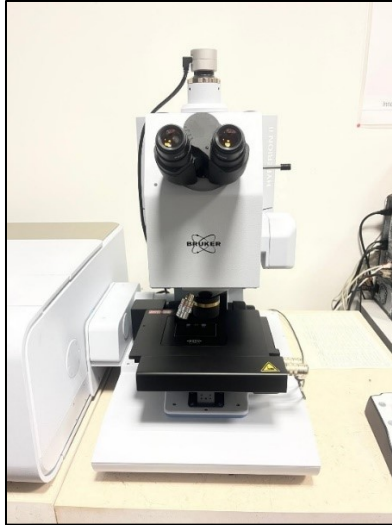
Figure 14: Bruker Hyperion II FTIR microscope located at the University of Padova, Department of Geosciences.
