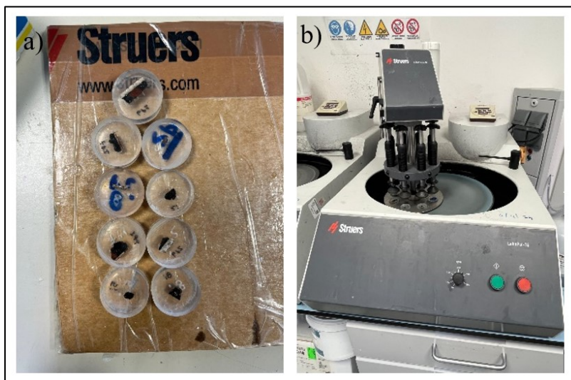
Figure 11: Left: unpolished samples embedded in resin. Right: Struers polisher.
