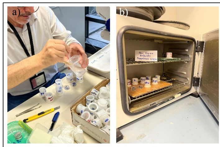
Figure 10: a) Plastic containers with samples being filled with epoxy resin. b) Sample containers in oven.
