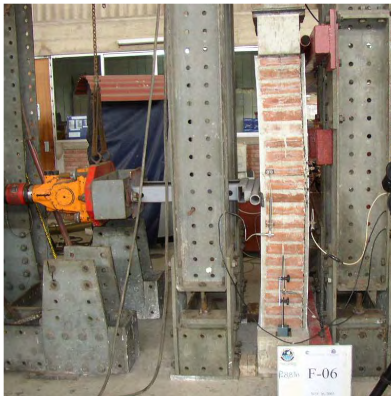
Fig. 3.19 – Grid reinforced wall submitted to out of plane bending
