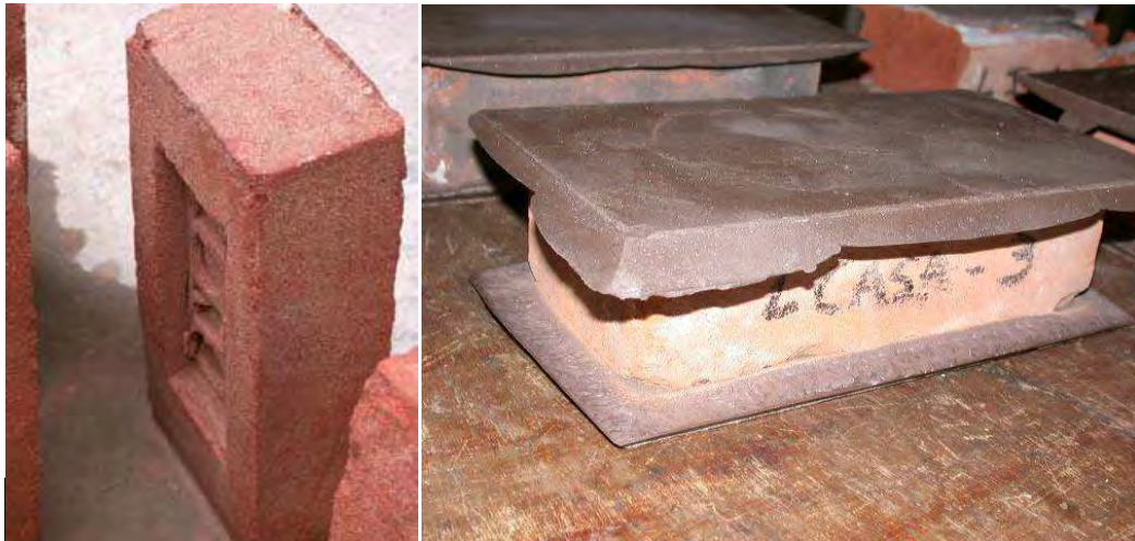
Fig. 2.1 – Brick units (a) and ready to be tested (b)
