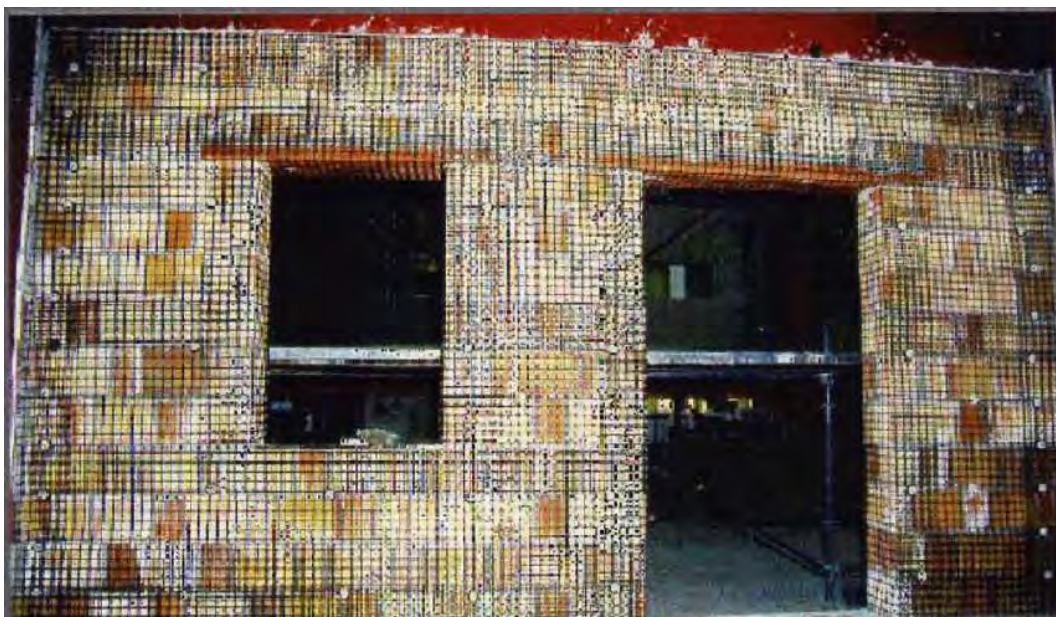
Fig. 3.17 – Wall with openings reinforced with polymer grid
