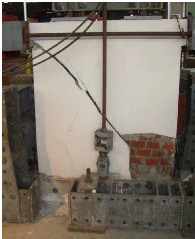
Fig. 2.23 – Diagonal crack formed during the shear – compression test
