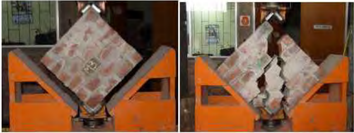
Fig. 2.4 – Diagonal compression test on wallets
