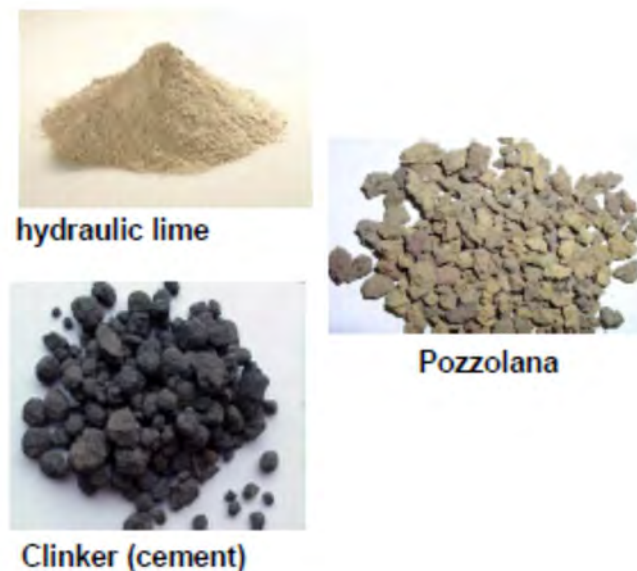
Fig. 1.2 - Type of binder of mortar
