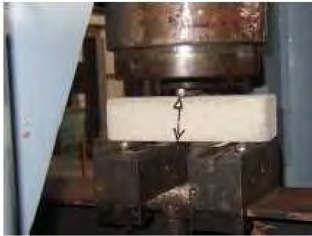
Fig. 2.2 – Flexure test of mortar sample
