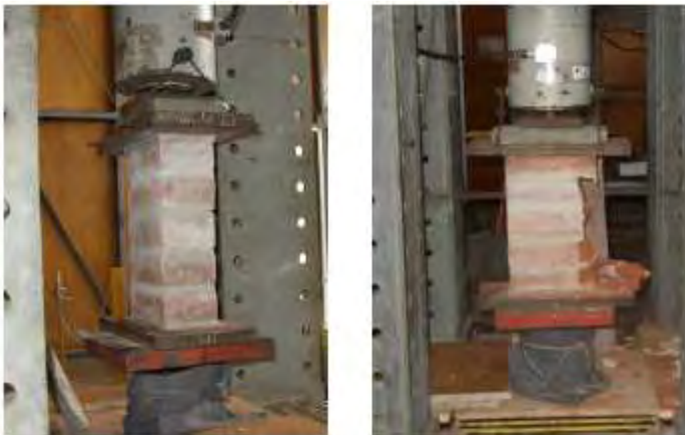
Fig. 2.3 - Compression test of masonry piles
