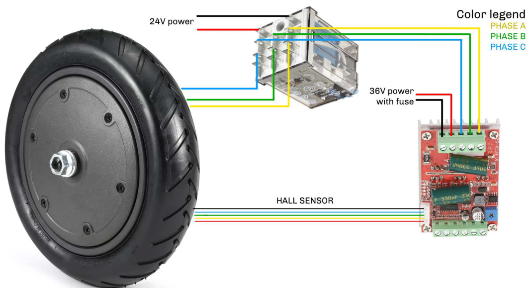
Figure 2.40: Schematic of the connection between each wheel with the motor driver.
