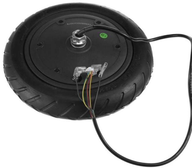
Figure 2.9: M365 250W 36V Motor Wheel Tire with Hall Sensor.
