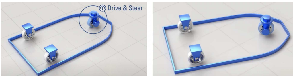
Figure 2.1: Steer drive system.
