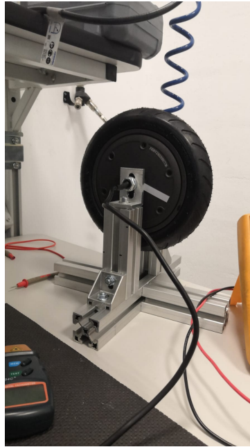
Figure 5.1: Work station used for testing the functioning of each BLDC motor wheel.
