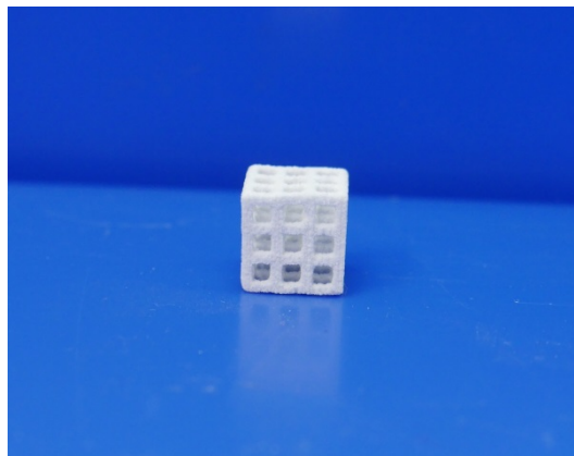
Fig.33b Scaffold printed with solution1 preparationA
