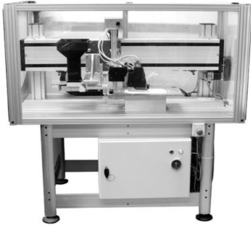
Fig.9a Powder based three dimensional printing machine used in this research
