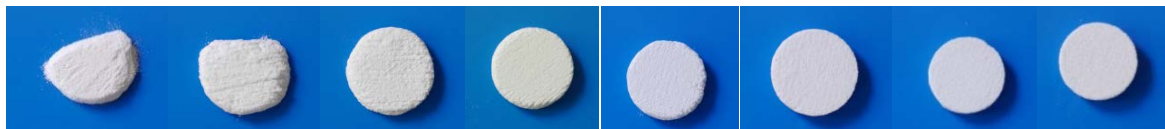
Sample1 Sample2 Sample3 Sample4 Sample5 Sample6 Sample7 Sample8 Table 20 Eight samples printed in order to discovered the right amount of solvent
