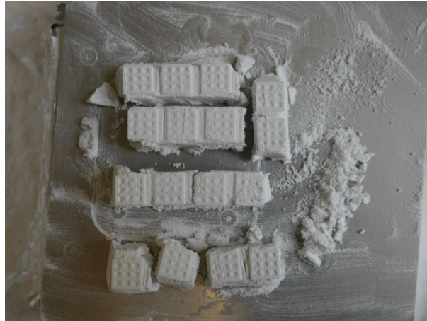
Fig.32 Scaffolds printed on the platform
