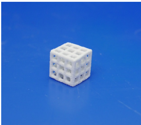
Fig.33a Scaffold printed with solution1 preparationA
