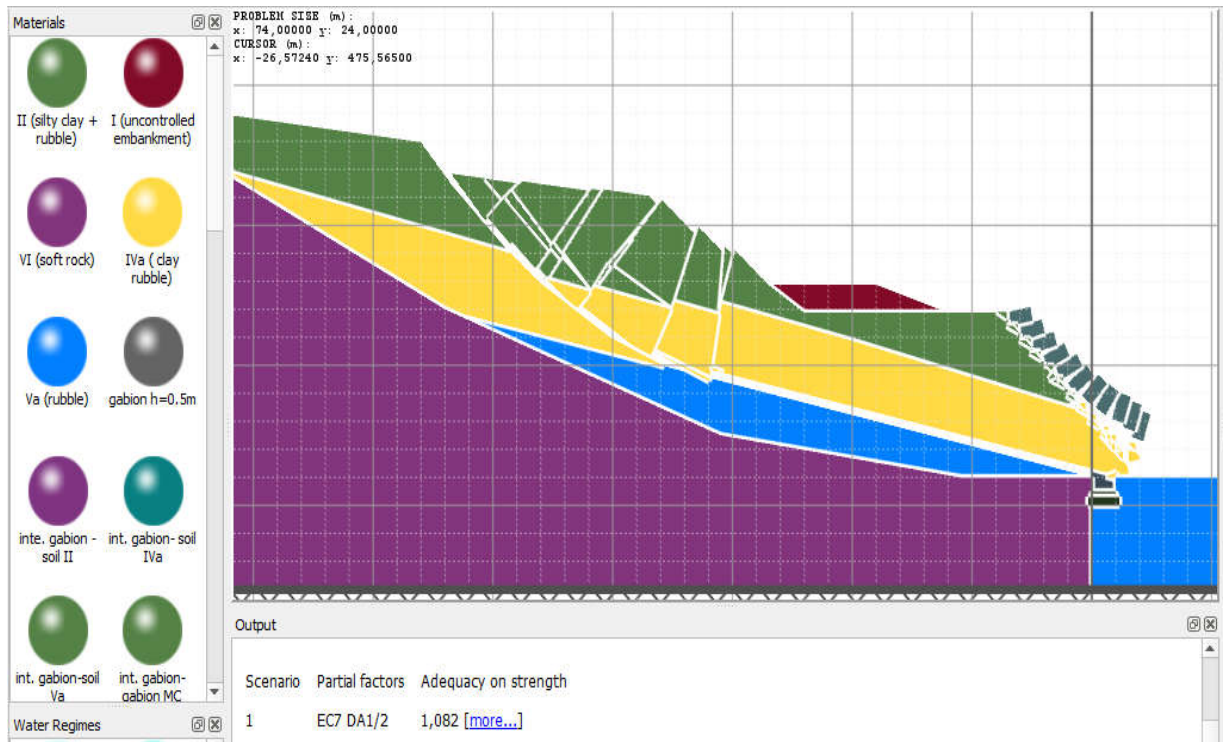
Figure 4.8. Failure mode of the landslide supported by gabions ( LimitState GEO 3.5 )
