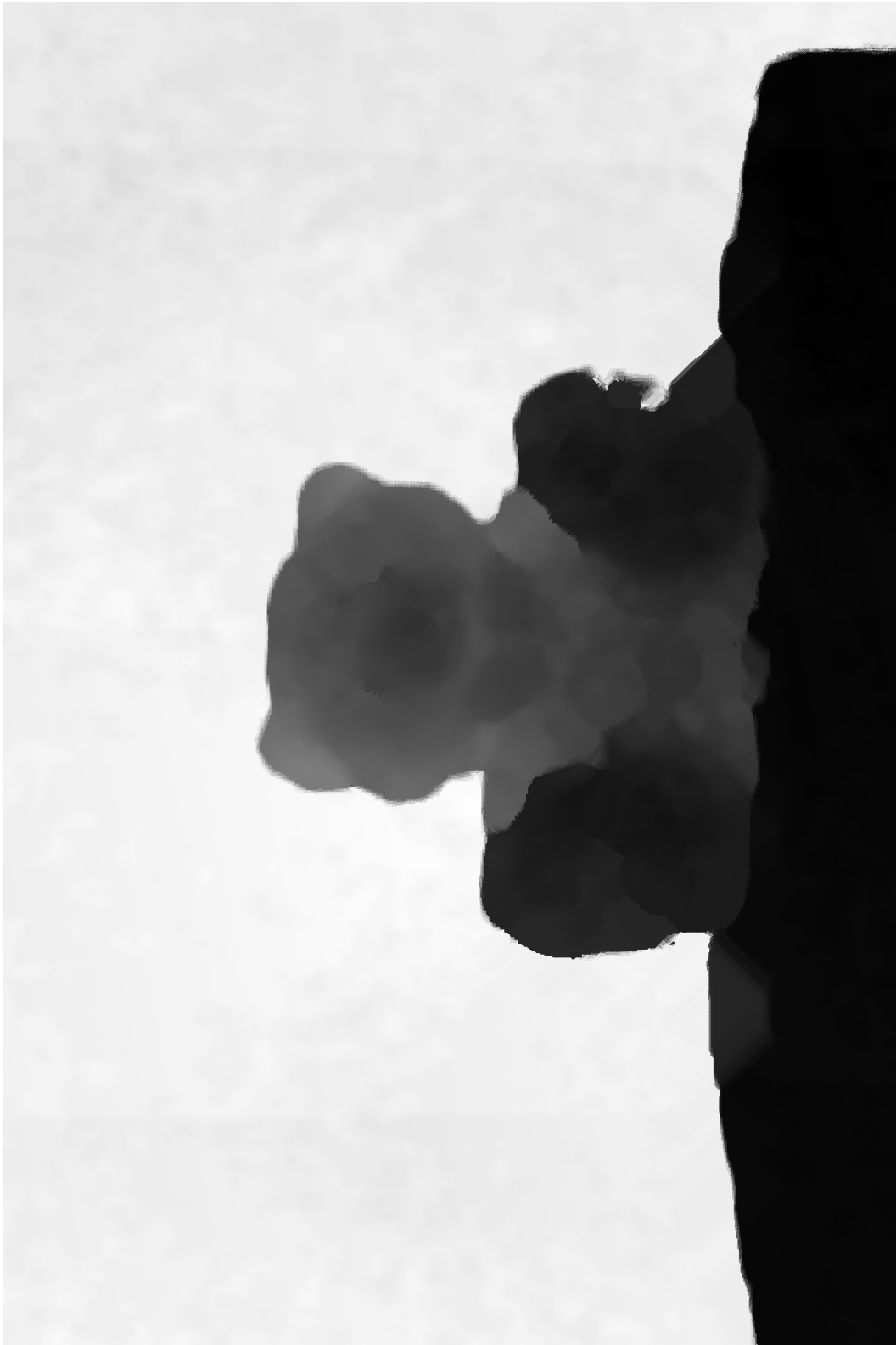
Figure 4.2: High resolution depth-map. It is the output of the trilateral filter algorithm.
