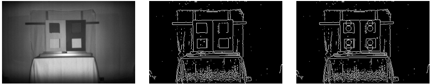
(a) Amplitude image from Canesta. (b) Canny computation for Canesta image. (c) Pixels detected for Canesta image.
