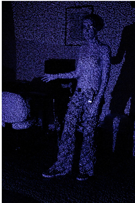
Figure 1.5: Structured light projection with dots.
