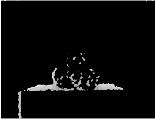
Figure 3.14: The result of radial smoothing operation for the pixels for which the depth is unknown.
