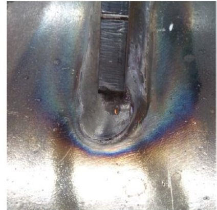
(a) As-welded local geometry
