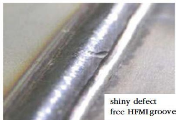
Figure 4. 8: a shiny and defect free HFMI groove [9].
