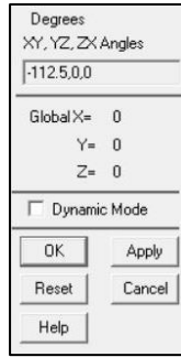
Figure 2. 14: work plane rotation by 112.5° clockwise about global z-axis.
