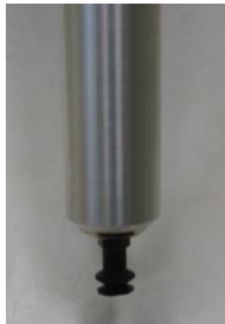
Figure 6.7: Vacuum cup (end effector).
