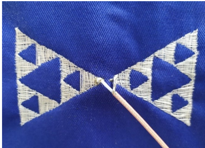
Fig 3.19: Hand embroidered bow tie antenna
