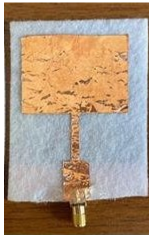
Fig 2.1: Patch antenna with copper conductive foil
