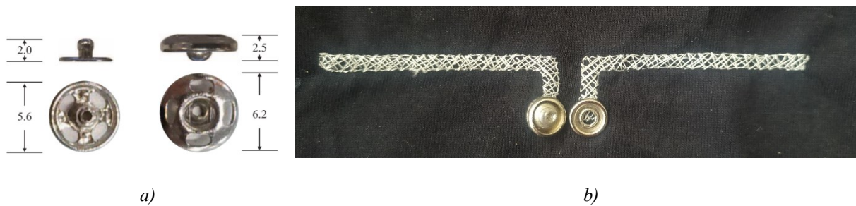
Fig 4.1: a) Snap fasteners b) Hand embroidered dipole antenna with snap fasteners
