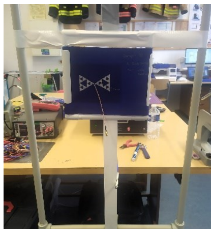
Fig 3.11: PVC structure to take measurements
