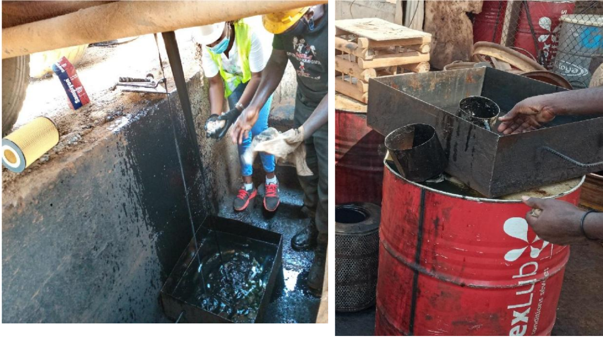
Fig 6: waste oil collection using metallic recipient and further transfer into 200L barren for storage using funnel and cup
