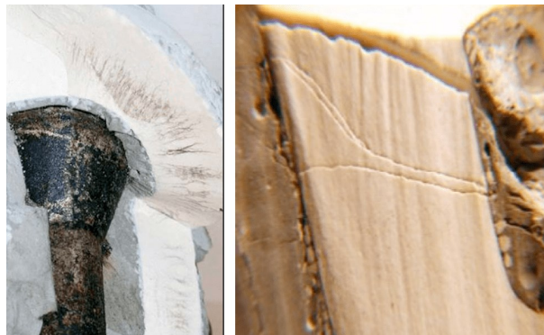
Figure 1.4. Internal punctures causing head cracking in porcelain insulators [3].
