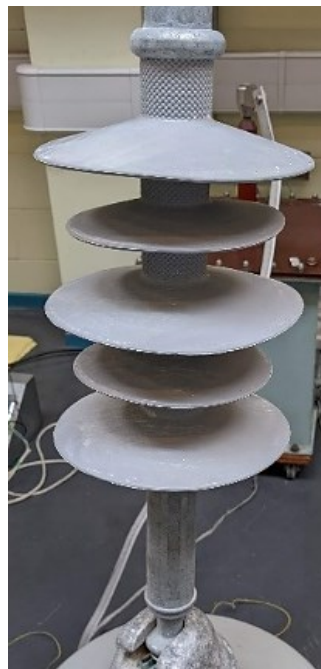
Figure 3.7. Textured silicon rubber insulator.
