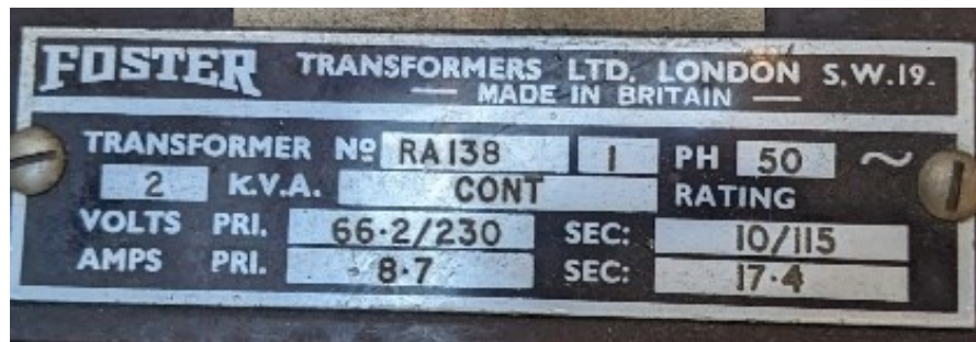
Figure 3.2. Foster isolation transformer 2 kVA, 230/115 V.
