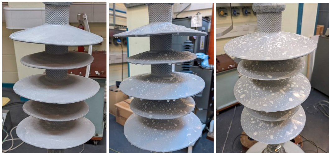
Figure 3.18. Starting from the left, there is the dry condition. In the centre the first wet pollution deposition and on the right the second spray of kaolin solution.
