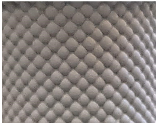
Figure 3.8. Shank pattern of the textured composite insulator.
