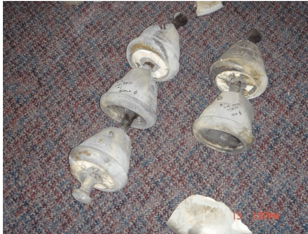
Figure 1.5. De-Capping of porcelain insulators [3].
