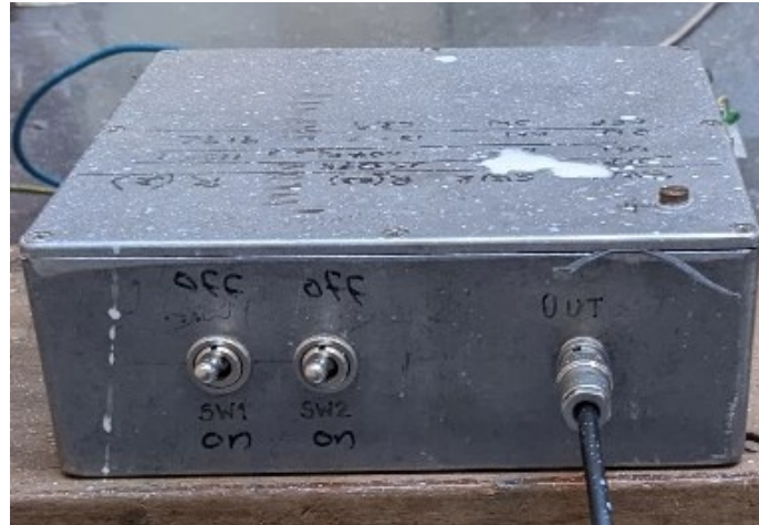
Figure 3.11. Shunt resistor box used for the test. With two switches, the Rbox had the possibility to change the R value from 91.92 Ohm to 4700 Ohm.
